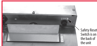
If the oil reaches 430°F (221°C) switch cuts power to the unit.
