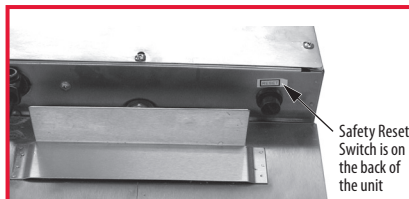
If the oil reaches 430°F (221°C) switch cuts power to the unit.
