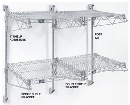
Adjustable Shelf Brackets allow you to adjust shelves on 1" increments. Shelves mount to posts individually or in as many tiers as needed. Choice of Single Shelf Bracket or Double Shelf Bracket. Use Double Shelf Bracket for assembling shelves in a continuous run. Double Shelf Bracket attaches to one post. Order one additional post kit for every 2 shelves. Post kit consists of 2 posts 4 wall brackets. Chrome finish.
