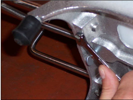
Figure 4. Pusher Head Adjustment Through the Blades.
